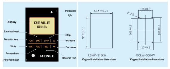
The keyboard panel can display English and Chinese. The keyboard panel has abundant functions, such as the keyboard panel running(frequency setting, running/stop command), function code data confirmation and change with many confirmation functions. Please operate the equipment after understanding the function operation completely. Indication lamp: Indicate the frequency inverter status.
